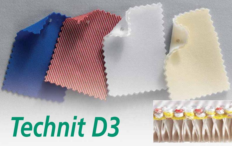
The Technit D3 is a new development from Mayer & Cie. which opens up totally new scope in circular knitting technology. It knits 3 threads on the cylinder side, two of which can be used as functional threads. The first plated thread is 50% visible on the face side (depending on the yarn used and machine setting), while the second plated thread is concealed in the centre of the fabric. This technology opens up totally new application possibilities for circular knitting factories.
